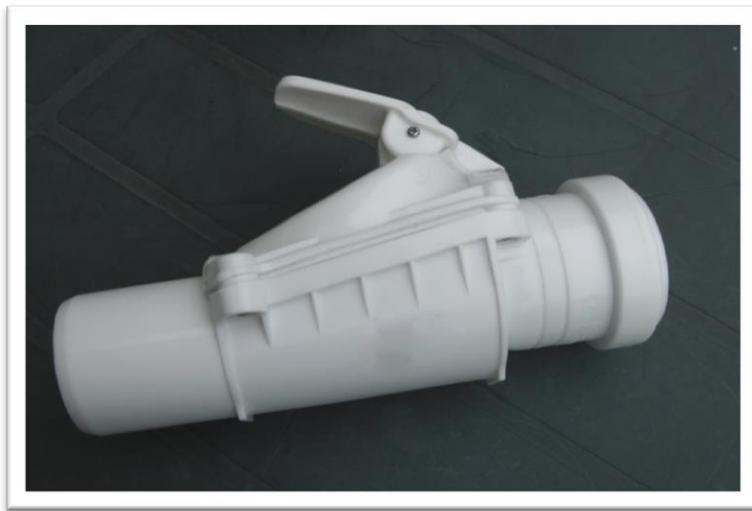
Back water valves allow water to flow in one direction. When water flows in the wrong direction a hinged flap automatically closes and stops water coming back into the home
